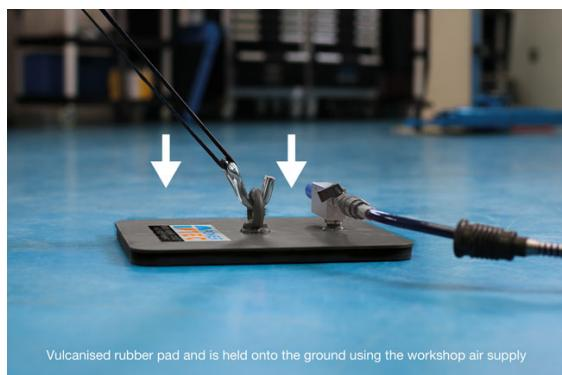
Vulcanised rubber pad and is held onto the ground using the workshop air supply
